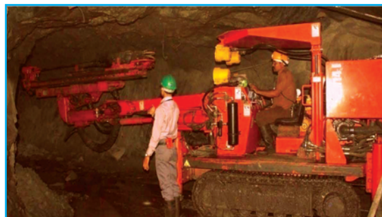
Underground Single Boomer Crawler Drilling Machine, installed at Balaghat Mine
