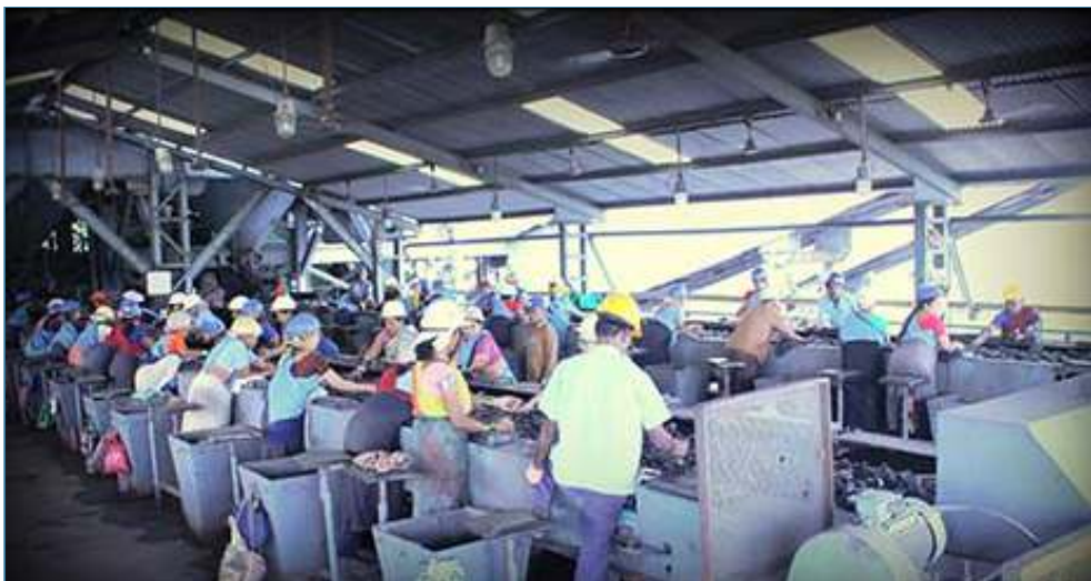
Picking Belt at IMP Plant
