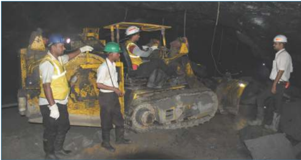
Side Dump Loader at MOIL's Mine
